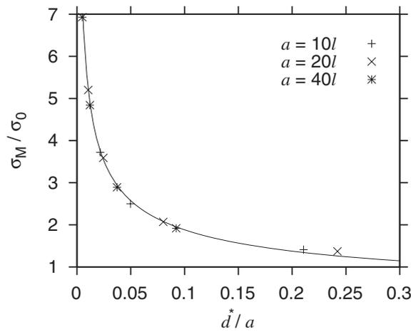
Fig. 5. The same plot with Fig. 4 but with renormalized quantities. The data for  $\epsilon = 1.0$  are collapsed onto a solid curve, or eq. (4) with  $\nu = -0.45$  (see Table I), when  $d^*/a \ll 1$ . The maximum stress in the system becomes smaller as the void size gets larger, following the scaling law indicated in the text.
