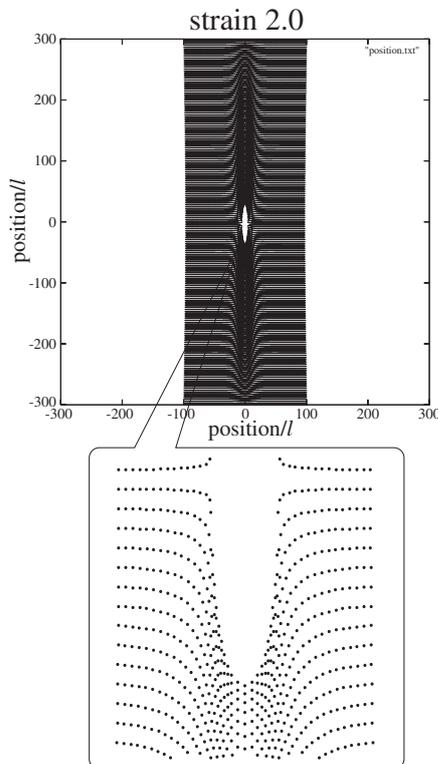
Fig. 2. Equilibrium positions of  $200 \times 200$ -point network with a crack ( $a = 20l$ ) when stretched to  $3L$  in the  $y$  direction. Positions are represented by small dots. A magnified view around the crack is shown at the bottom.
