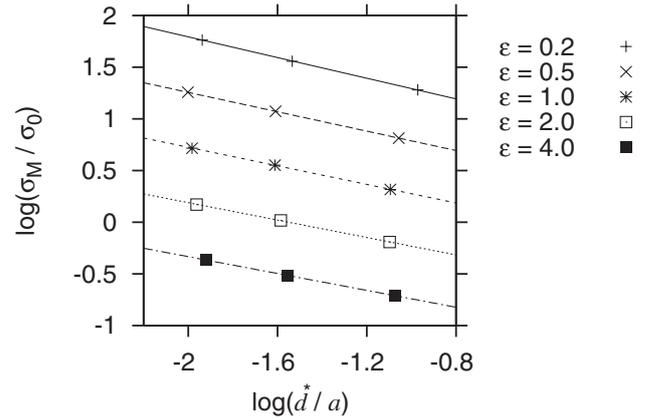
Fig. 7. Relation between  $\sigma_M$  and  $d^*$  for three smallest values of  $d^*/a$  at different strains from  $\epsilon = 0.2$  to  $4.0$  for a given crack length  $a = 20l$ . The points for  $\epsilon = 0.2, 0.5, 2.0$ , and  $4.0$  are shifted by  $1.0, 0.5, -0.5$ , and  $-1.0$  upwards, respectively, to avoid overlap. The slope slightly depends on strain as stipulated in Table I.
