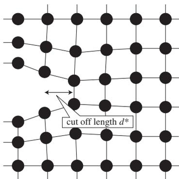
Fig. 6. The cut-off length  $d^*$  is identified with the smallest length scale appearing in the numerical calculation: the  $x$ -coordinate difference between the tip and its nearest neighbor.
