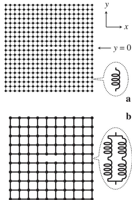
Fig. 1. Illustration of the present models for materials with voids for a small  $N$  and  $m$  ( $N = 20, m = 2$ ): (a) the original network system and (b) another system with the double mesh size. In (b), a bundle of two serial connections of two original springs in (a) are used to connect the points, to obtain the identical bulk elasticity. Crack size ( $a = 6l$ ) is the same in the two systems.
