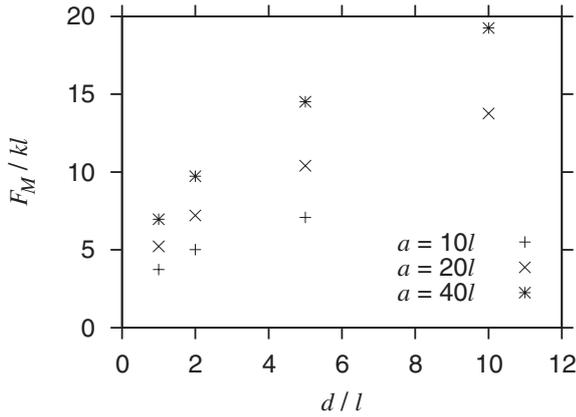
Fig. 4. Change of the maximum force  $F_M$  at the tip with void sizes  $d$  for a given stress  $\epsilon = 1.0$  and a given system size ( $N = 200$ ). Three crack sizes,  $a = 10l$ ,  $20l$ , and  $40l$ , are examined.
